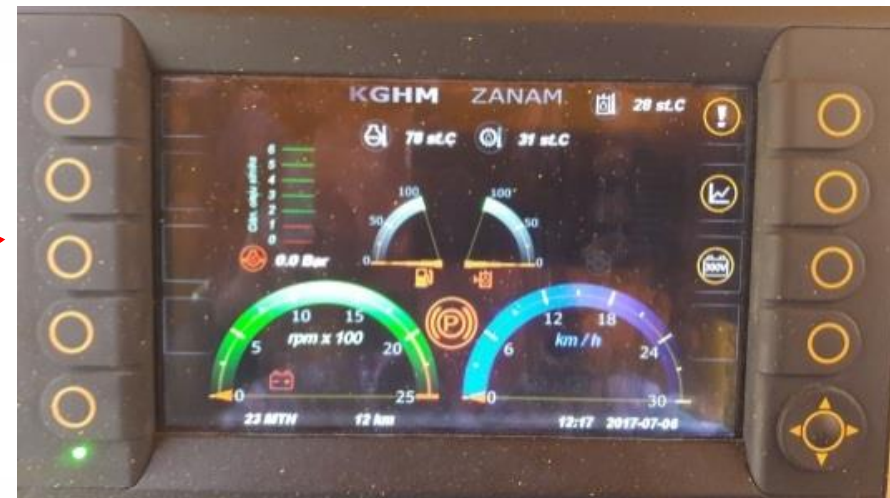
Battery unit working parameters display.
