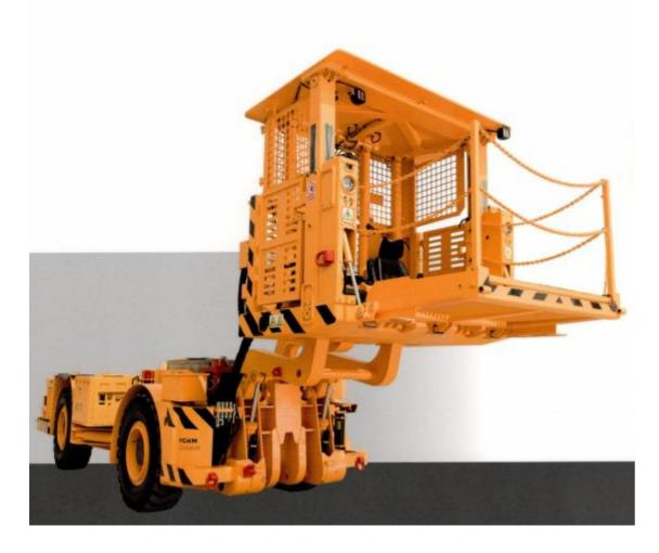
Mobile Pumping Unit MUP-4 produces bulk emulsion explosives from matrix and sensitizer directly during the loading into boreholes in the mine.
