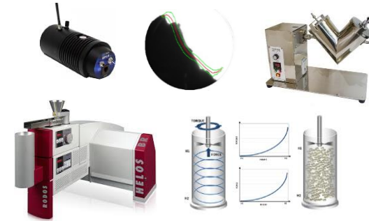
Powder characterization and preparation: PSD, FT4 rheometry, laser absorption, flowability, V-shape mixer, mechanical alloying drum etc.
